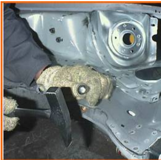
Figure 2.3 Pry checks are routinely performed on spot-welded steel assemblies to ensure the quality of the welds.
