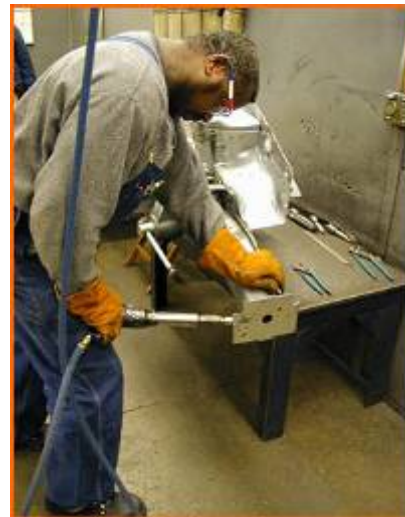
Figure 2.4 Full body-in-white teardowns are performed periodically, during which every welded joint is pried apart to examine and measure the resulting weld buttons.
